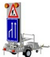
Advance warning trailers
