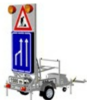
Advance warning trailers
